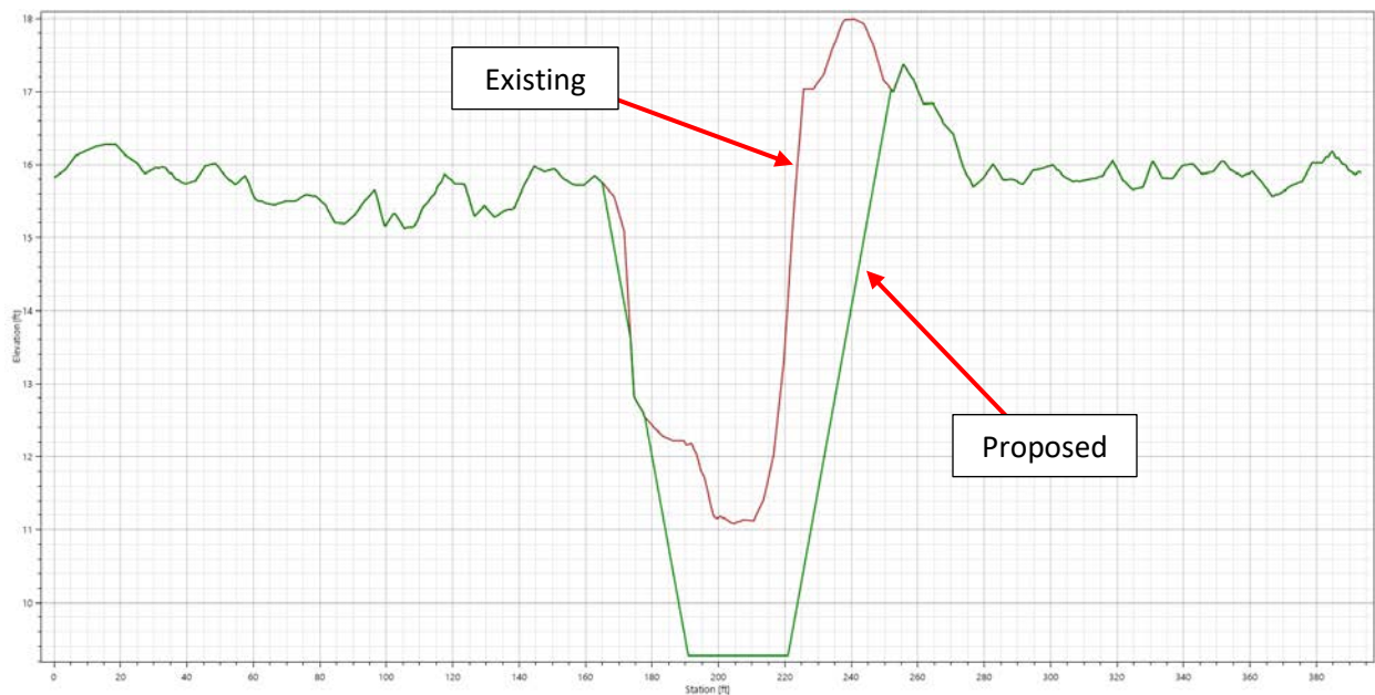
Figure 13: Typical cross section improvement
